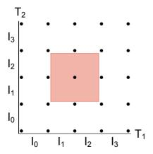
A critical section can be marked on a progress graph.
