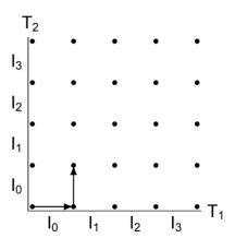
Each point marks the completion of an instruction in one thread
